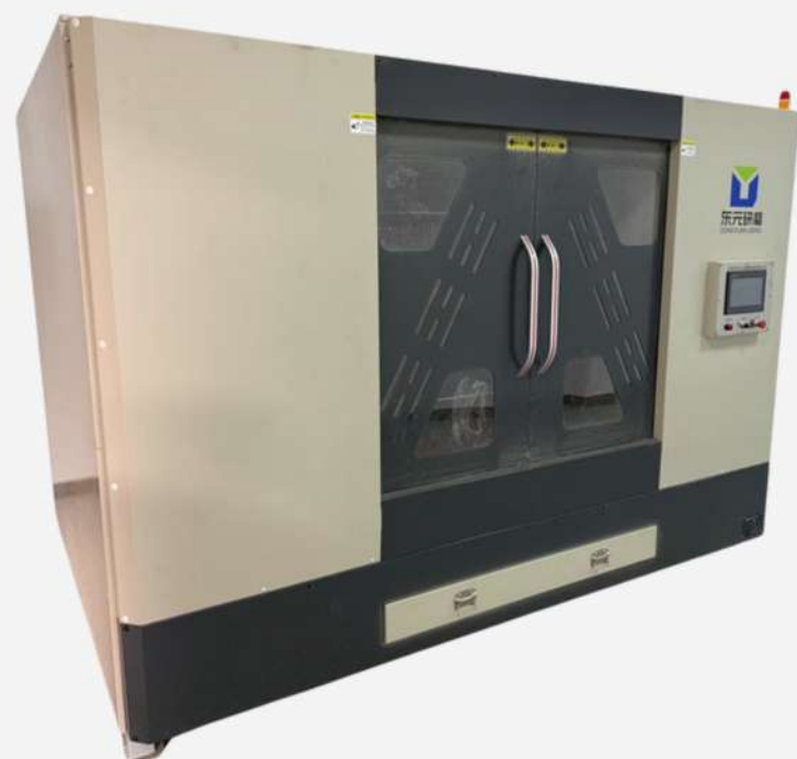
AUTOMATIC POLISHING MACHINE (METAL)
