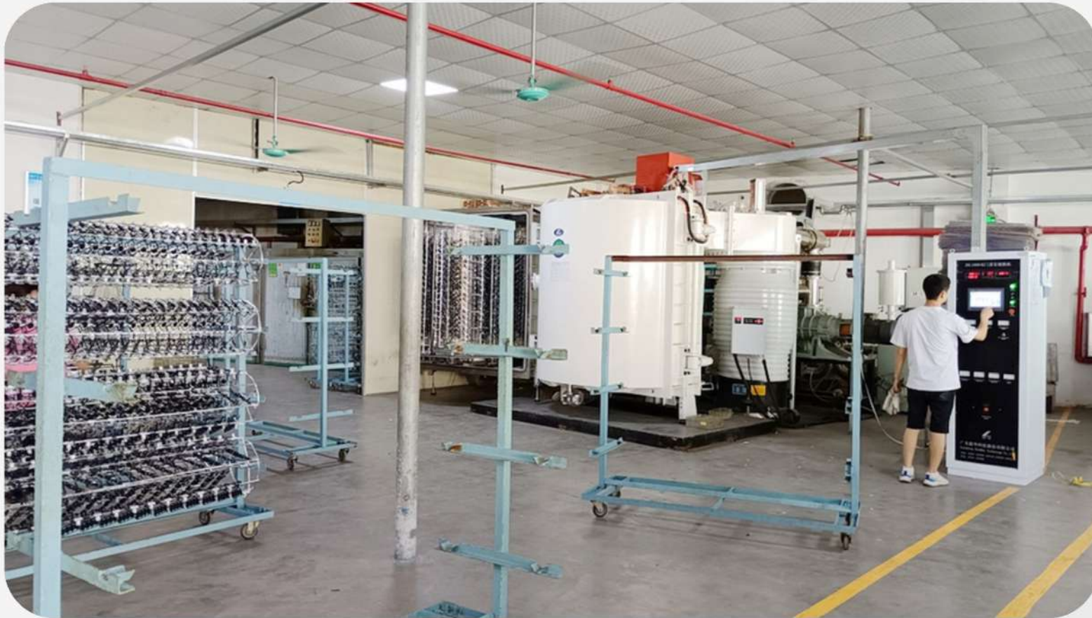
VACUUM PLATING / PHYSICAL VAPOR DEPOSITION (PVD)
